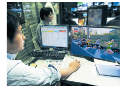
New presentation using computer graphics through automatic estimation of distances between runners by applying image recognition AI technology
